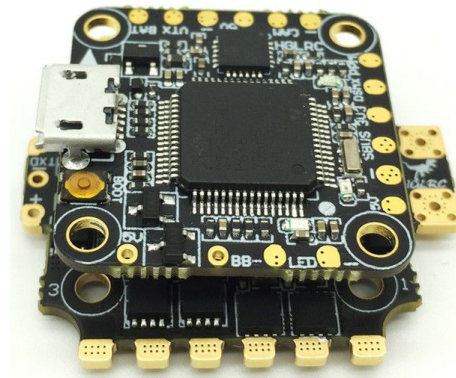
Figure 116: HGLRC F440 FC with 40A BLHeli 32 4-in-1 ESC
