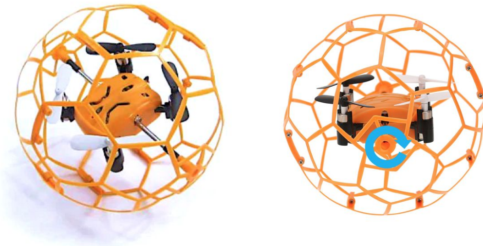
Figure 102: Example of mesh-enclosed UAV
