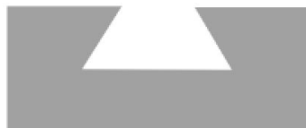
Figure 101: Cross section of track for spring-propelled cart
